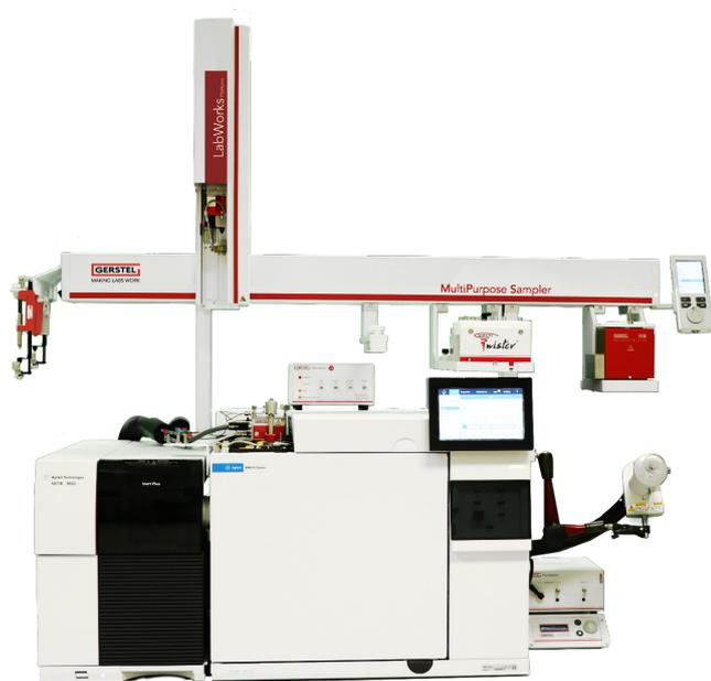
**Figure 1:** MPS LabWorks Platform equipped with ODP 4 used in this study.
