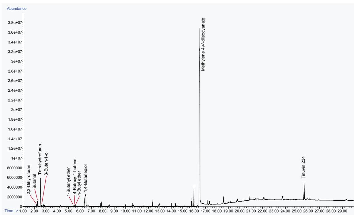
**Figure 4:** Total ion chromatogram for pyrolysis of a disc sample containing polyurethane.
