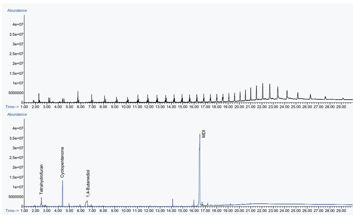
**Figure 6:** Stacked view of total ion chromatograms for pyrolysis of two discs from the same manufacturer.
