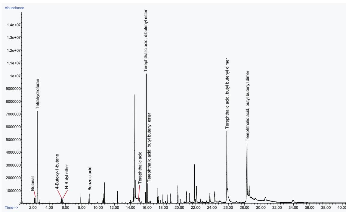
**Figure 2:** Total ion chromatogram for pyrolysis of a disc sample.
