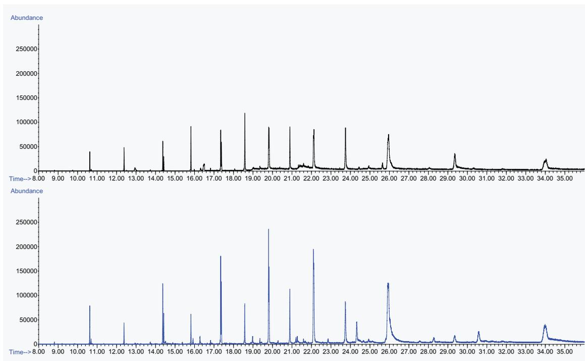
**Figure 5:** Extracted ion chromatograms ( $m/z=129$ ) for the polyurethane sample (top) and polyester sample (bottom).
