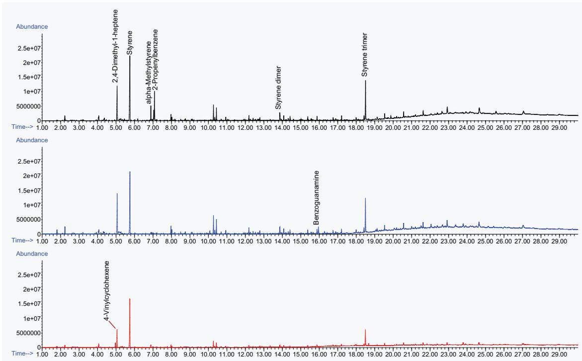
**Figure 3:** Stacked view of three total ion chromatogram for pyrolysis of three disc samples containing polystyrene/polypropylene.
