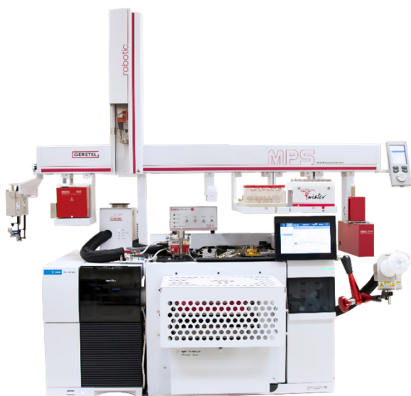
Figure 1: Selectable ^1\text{D}/^2\text{D} -GC-MSD system (optional ODP and DHS shown).
