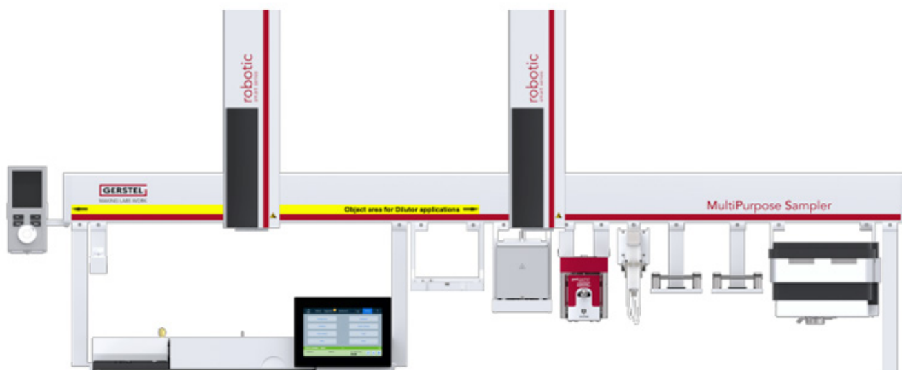
Figure 2: Analysis system used for automated determination of 3-/2-MCPD- and glycidol-esters from edible oils and fats according to ISO 18363-4. The MultiPurpose Sampler (MPS) mounted on top of the GC-MS/MS performs all sample preparation steps. The heads are equipped with a 10 \mu L syringe for sample injection (left) and a 1 mL syringe for sample preparation (right). From left to right the modules included are: 10 mL wash station, tray holder for sample/extract vials, agitator, a quickMIX module high power agitator, a high flow fast wash station, several 180 mL solvent reservoirs and cool-tray.
