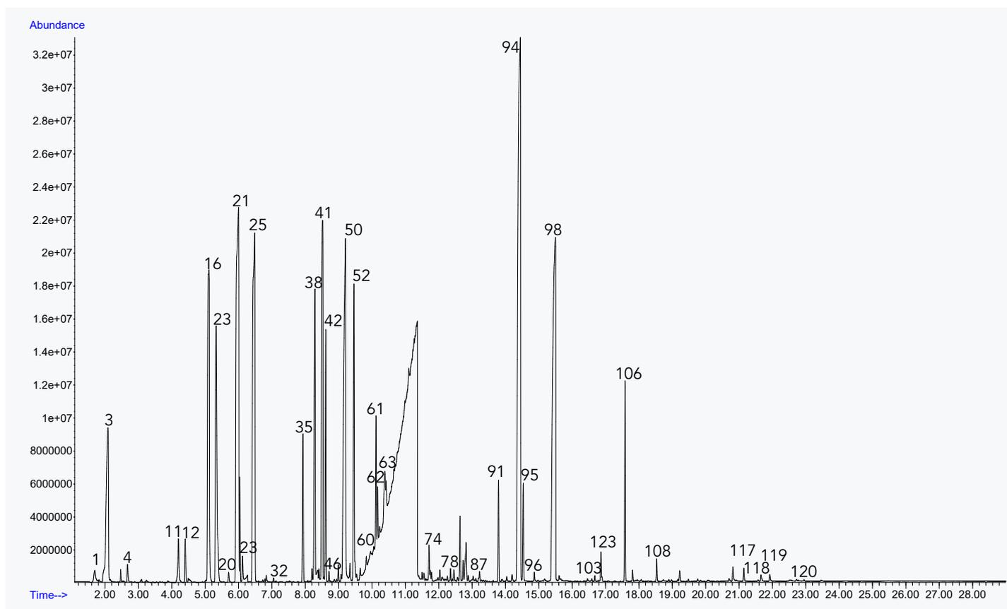
**Figure 4:** Total ion chromatogram obtained for the undiluted watermelon hard seltzer using the simultaneous extraction technique with a 20:1 split transfer.
