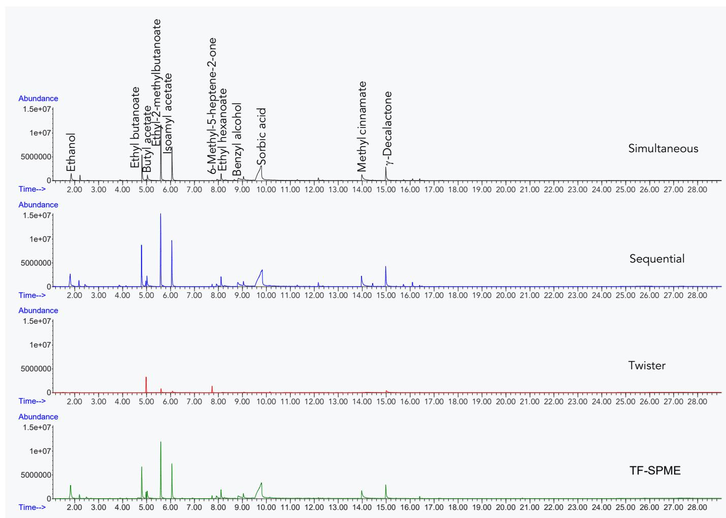
**Figure 2:** Stacked view of total ion chromatograms obtained for the watermelon hard seltzer using the simultaneous (top), sequential (top middle), Twister® stir bar (bottom middle), and PDMS/HLB TF-SPME extraction techniques (bottom).
