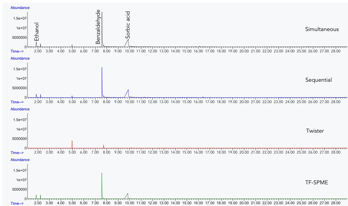
**Figure 1:** Stacked view of total ion chromatograms obtained for the black cherry hard seltzer using the simultaneous (top), sequential (top middle), Twister<sup>®</sup> stir bar (bottom middle), and PDMS/HLB TF-SPME extraction techniques (bottom).
