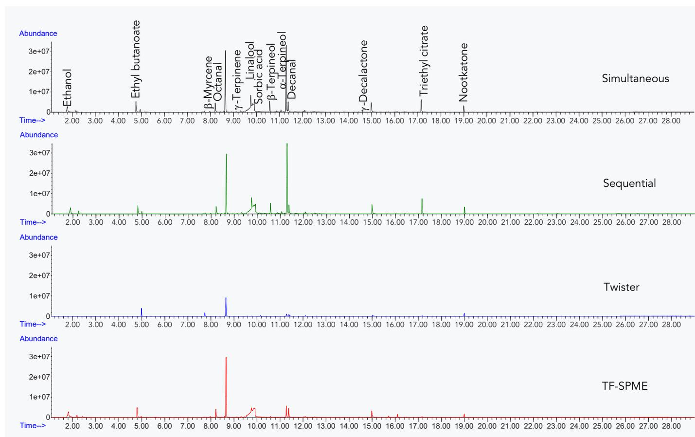
**Figure 3:** Stacked view of total ion chromatograms obtained for the grapefruit hard seltzer using the simultaneous (top), sequential (top middle), Twister<sup>®</sup> stir bar (bottom middle), and PDMS/HLB TF-SPME extraction techniques (bottom).
