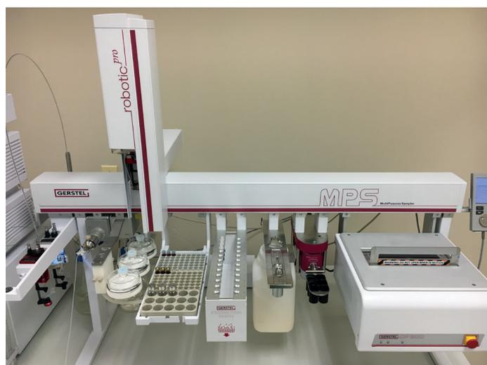
**Figure 1:** MPS robotic<sup>PRO</sup> sampler with GERSTEL quickMIX and CF-200 centrifuge options.
