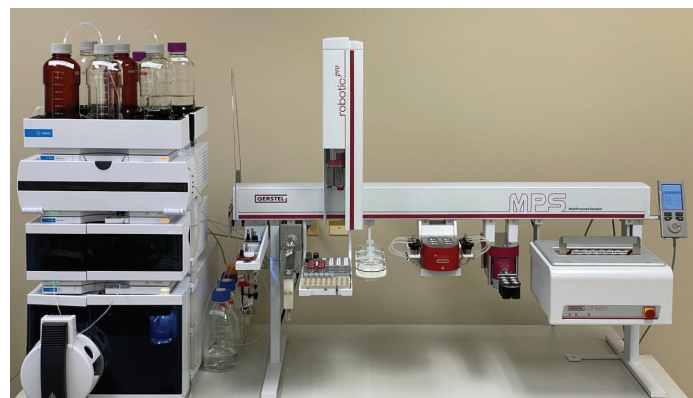
Figure 1: MPS robotic PRO sampler with GERSTEL quickMIX, mVAP, and CF-200 centrifuge options.
