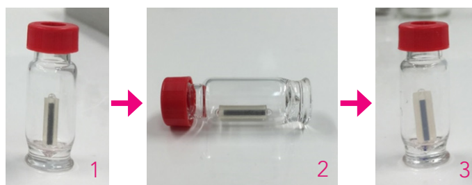
Figure 1: FLEX-Twister and solvent swelling procedure.
