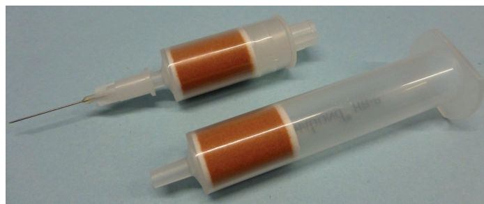
Figure 2: Top: Standard solid phase extraction (SPE) cartridge adapted for automated SPE with the GERSTEL MPS. Such cartridges are commercially available from a number of vendors. Bottom: standard solid phase extraction cartridge.
