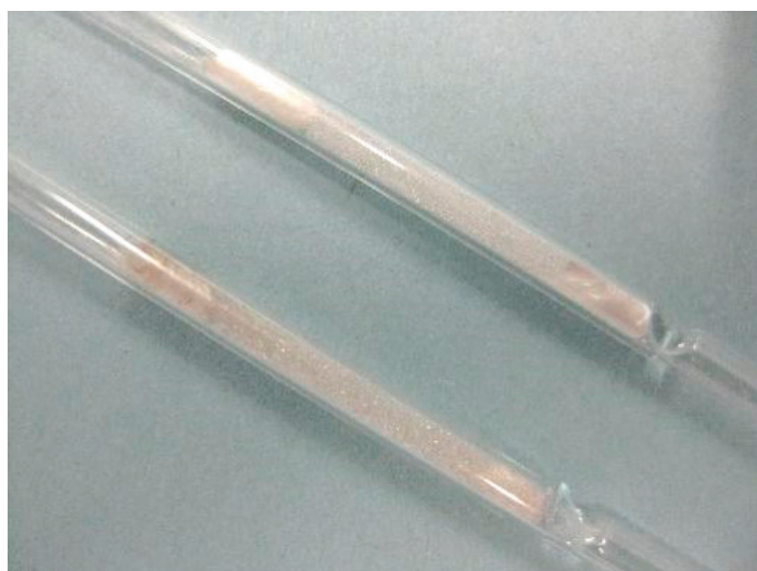
Figure 16: CIS GC inlet liner new (top) and after >50 samples (bottom). Due to effective sample cleanup, the used inlet liner is relatively clean.
