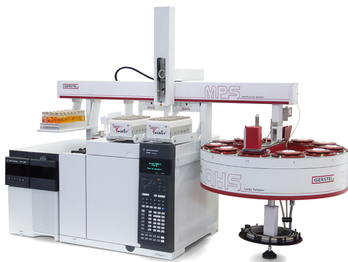
Figure 1: 11-Position on-line micro-scale chamber system combined with GERSTEL LabWorks Platform and coupled with GC/MS.
