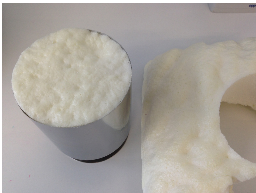
Figure 3: Custom-made coring tool and sample of the SPF open-cell foam (left) and the coring tool together with the sample, the surface at the top, placed into the one Liter container (right).
