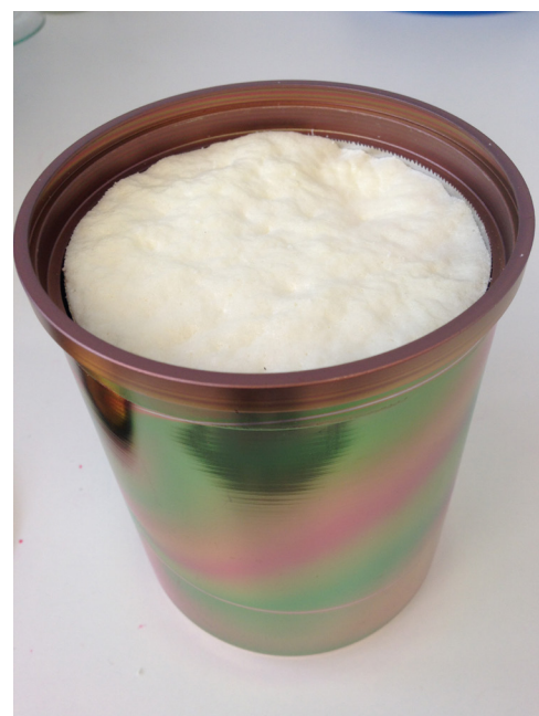
Figure 3: Custom-made coring tool and sample of the SPF open-cell foam (left) and the coring tool together with the sample, the surface at the top, placed into the one Liter container (right).
