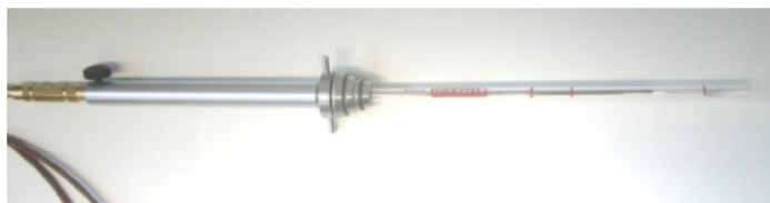
Figure 9: Adapter for sample area true temperature measurement in the TDS 3.
