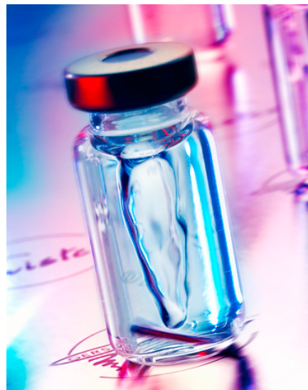
Figure 1: The GERSTEL Twister® stirring and extracting a liquid sample.
