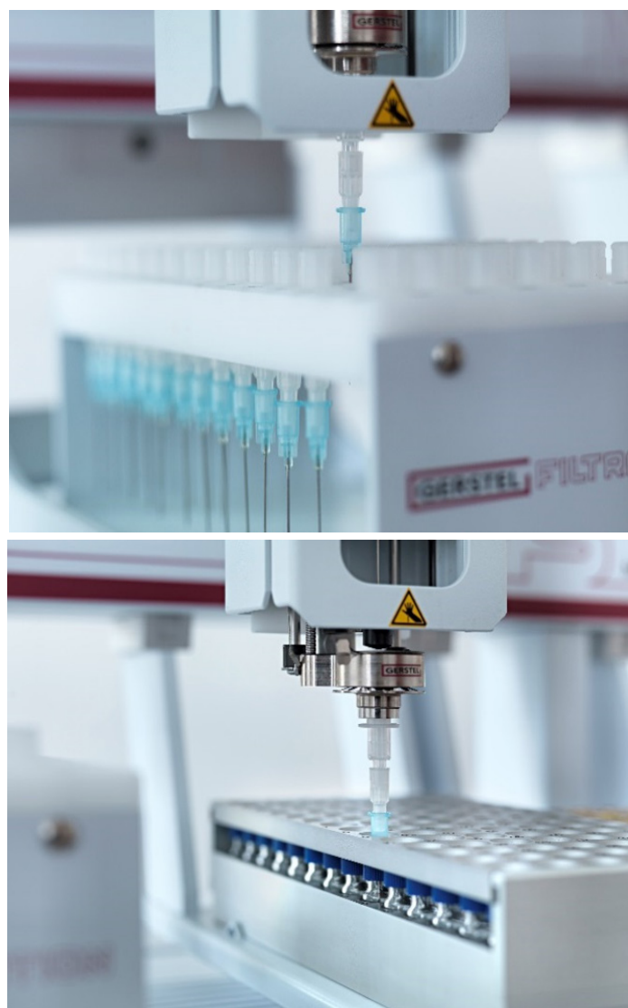
Figure 3: Pictures of the MPS transporting the 0.45 \mu\text{m} filter from the filtration tray (top) to the VT-98 tray with filtration cover (bottom).
