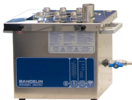
Figure 2: Picture of the ultrasonic bath used for automated ultrasonic extraction of the plant material.
