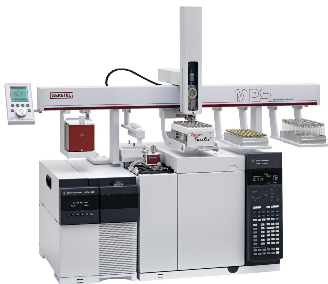
Figure 1: GC/MS system for thermal desorption of edible oils: GERSTEL LabWorks Platform on Agilent GC 7890 / MSD 5977.
