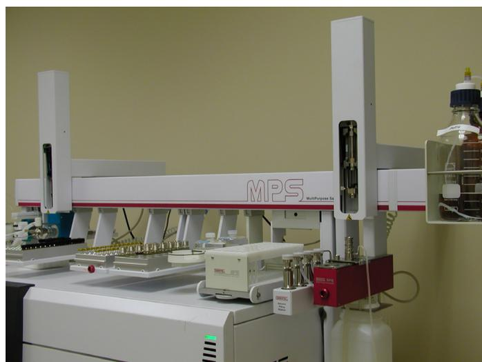
**Figure 2:** MultiPurpose Sampler (MPS XL) with GERSTEL SPE Option.
