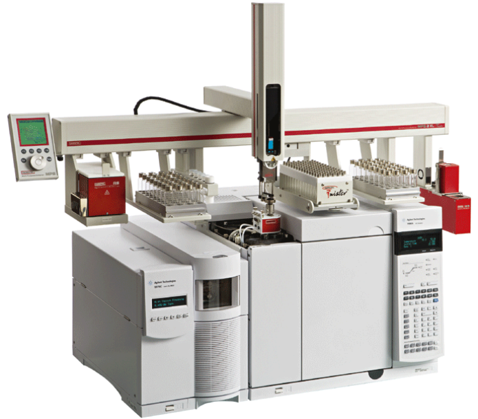
Figure 1. GERSTEL LabWorks Platform with DHS option on an Agilent Technologies 7890 GC / 5975 MSD.
