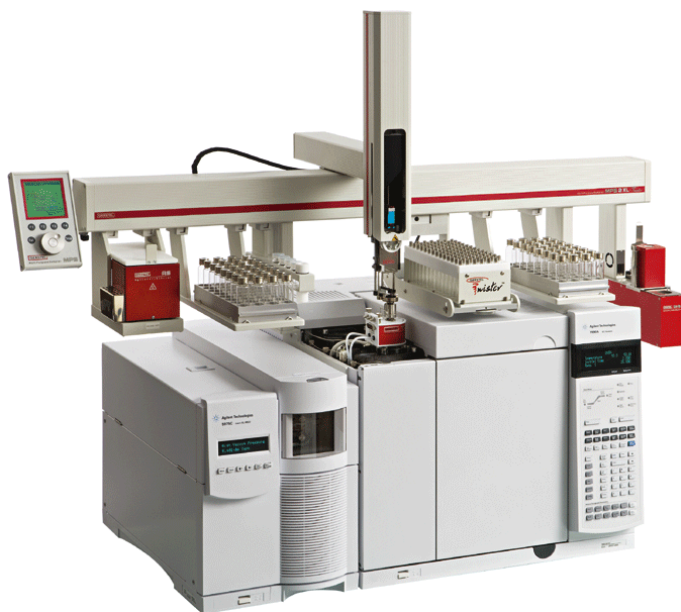
Figure 2: GERSTEL LabWorks Platform with DHS option mounted on an Agilent Technologies 7890 GC / 5975 MSD.
