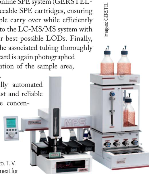
MPS-based GERSTEL DBSA Autosampler (to the left) with SPE<sup>nos</sup>-Module (right hand side) for direct connection to the LC-MS/MS system (not shown).
