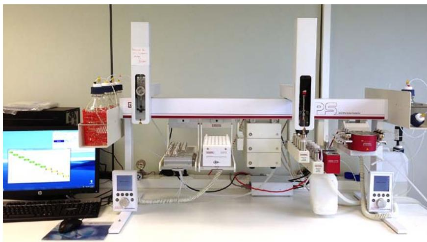
Figure 1. MPS Dual Head WorkStation configured for automated SPE and analyte concentration.
