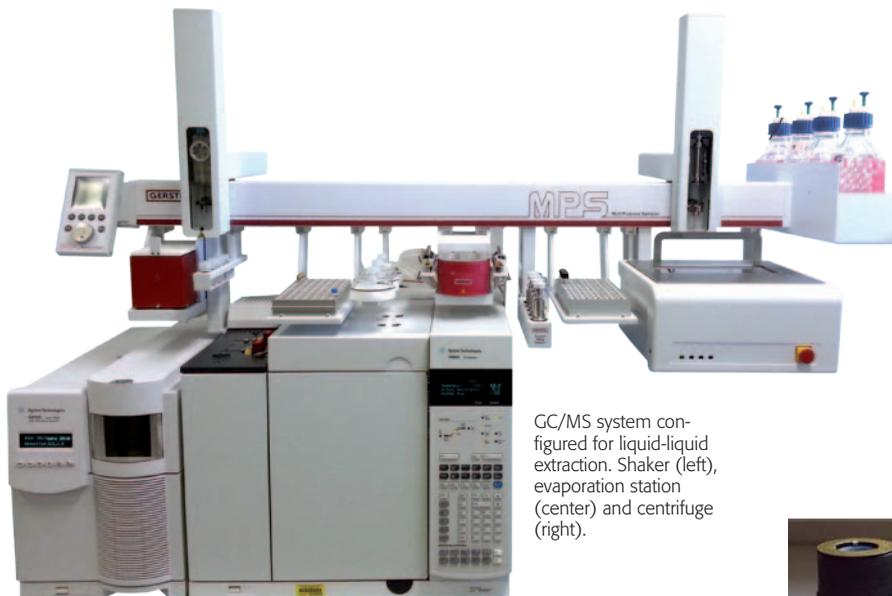
GC/MS system configured for liquid-liquid extraction. Shaker (left), evaporation station (center) and centrifuge (right).
