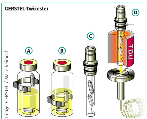
Figure 1: Schematic diagram of the multi stir bar extraction process using Twicester® (A) Magnetic positioning of up to three Twisters using Twicester Showing 1 Twister in HS & 1 stirring (B) HSSE using two Twisters submerged in liquid (C) Transfer of Twisters to TDU Tube (D) Simultaneous thermal desorption of the Twisters, cryofocusing in the CIS and GC/MS analysis.
