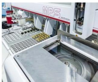
GERSTEL MultiPurpose Sampler (MPS) equipped with centrifuge, *m*VAP and *quick*Mix.
