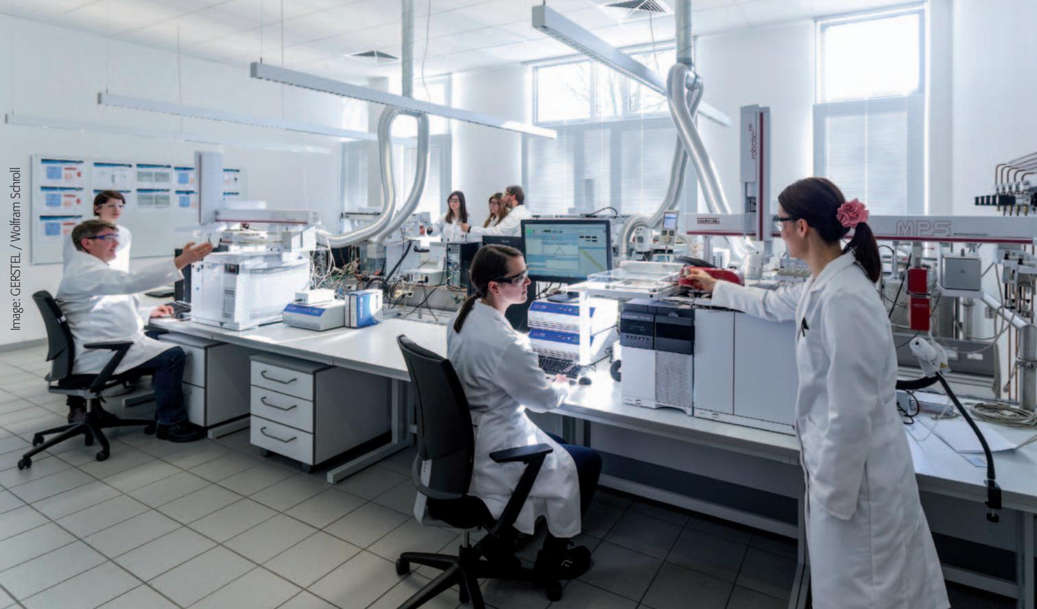
A modern GC/MS Laboratory. The analysis systems are equipped with high performance autosamplers that can automate all steps in sample preparation and introduction. The high degree of automation helps ensure productivity and throughput while offering enough flexibility to easily adapt to new sample types, analysis methods and performance requirements.
